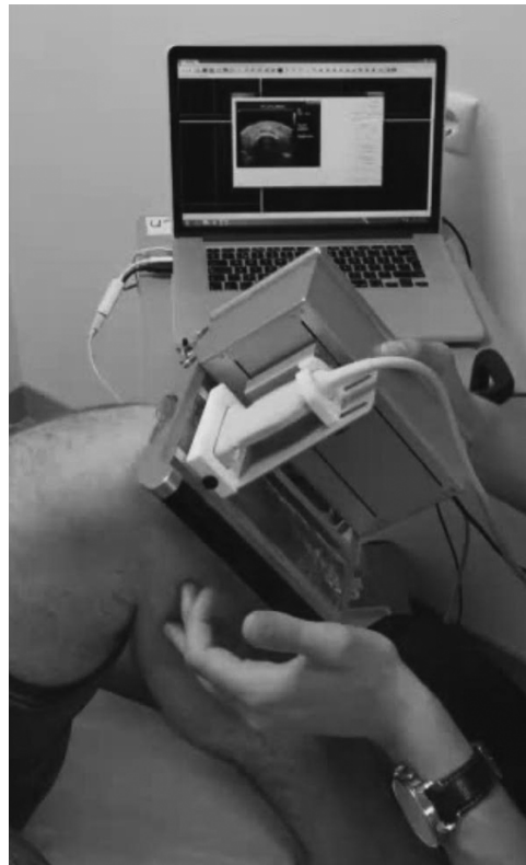
Fig. 1. Setup of ultrasound tissue characterization scan of the patellar tendon.
